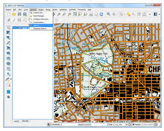
6. Select the Digitizing tab in the Options dialog. Set the Default snap mode to To vertex and segment. This will allow you to snap to the nearest vertex or line segment. I also prefer to set the Default snapping tolerance and Search radius for vertex edits in pixels instead of map units. This will ensure that the snapping distance remains constant regardless of zoom level. Depending on your computer screen resolution, you may choose an appropriate value. Click OK.
